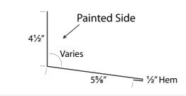
STEP SIDEWALL FLASHING
